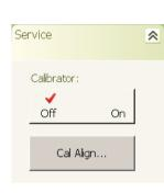
**Calibrator:** To toggle the internal 50 MHz calibrator Off or On, press on the calibrator Off/On toggle button.
