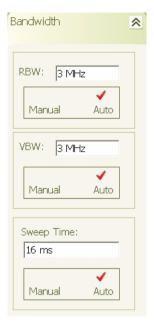
**2.** Select Auto VBW mode or press in the VBW parameter field and use the keypad to enter the desired bandwidth, then select the appropriate terminator from the fly-out menu.
