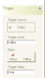
**Trigger Source:** To change the trigger source, press on the Trigger Source button and select the trigger source from the fly-out menu selections listed under Trigger Level below:
