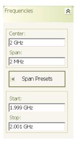
**2.** Press in the Center parameter field and use the keypad to enter the desired center frequency, then select the appropriate frequency terminator from the fly-out menu.
