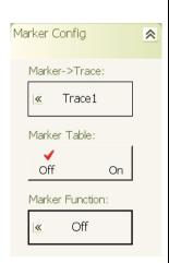
**Marker -> Trace:** To select the trace that receives the marker, press on the Marker On Trace field and select the trace from the fly-out menu.
