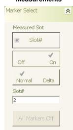
When in the WCDMA measurement mode with the Transmit Power Control graph type selected, the following marker selections are available (Refer to the WCDMA Graph Type Dialog on page 4-48 for information on setting graph types):
