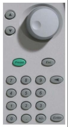
**Increment Up/Down:** Use the increment up/down keys to increment an active parameter (up or down) and to move an active marker to the next step. The increment up/down keys allow you to increment or decrement the active parameter in coarse/discrete steps. These steps usually follow the 1, 2, 3, 5 convention. These keys are mapped to the Page Up/ Page Down keys on a standard keyboard.
