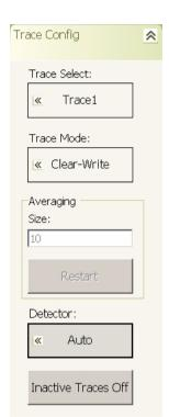
**Trace Select:** To set the active trace, press on the Trace Select button and select the active trace from the fly-out menu. When a trace is selected, the current trace mode is Off unless it was previously defined.
