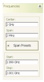
2. Press in the Span parameter field and use the keypad to enter the desired frequency span, then select the appropriate frequency terminator from the fly-out menu.
