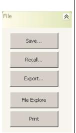
To save the current instrument setup, press on the Save... button to open a Windows Save As dialog. You can enter a name for your current setup and save the file as an Anritsu Setup File (.asr). The current default folder is C:\Signature\Setup\.
