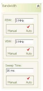
**2.** Select Auto RBW mode or press in the RBW parameter field and use the keypad to enter the desired bandwidth, then select the appropriate terminator from the fly-out menu.
