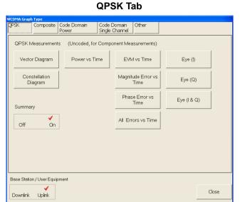
For QPSK measurements, the following graph types can be selected:
