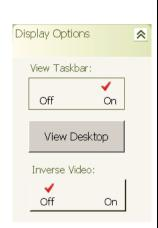
View Taskbar: To display the Windows taskbar, press the View Taskbar toggle button.
