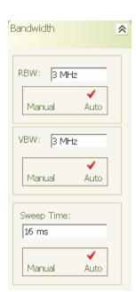
**RBW:** To change the resolution bandwidth when in the manual mode, press in the RBW parameter field and enter a new value using the numeric keys. When a new value is entered, the terminator fly-out will appear with the available units. Press on the desired units to terminate the entry.
