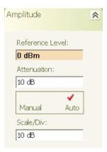
**2.** Press in the Reference Level parameter field and use the keypad to enter the desired reference level, then select the appropriate amplitude terminator from the fly-out menu.
