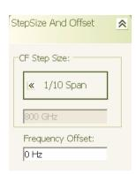
**CF Step Size:** To set the center frequency step size, press the CF Step Size button and select the desired step size from the fly-out menu.
