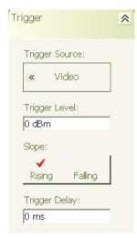
2. To change the trigger source, press the Trigger Source button and select the trigger source from the flyout menu below:
