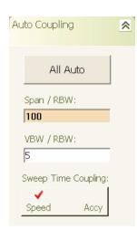
To select the fully coupled mode, press the All Auto button. This couples all of the bandwidth coupling factors automatically.
