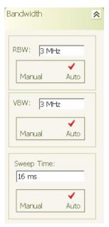
**2.** Select Auto Sweep Time mode or press in the Sweep Time parameter field and use the keypad to enter the desired sweep time, then select the appropriate terminator from the fly-out menu.
