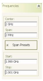
**2.** Press in the Start parameter field and use the keypad to enter the desired start frequency, then select the appropriate frequency terminator from the fly-out menu.
