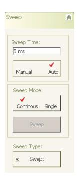
**Sweep Time:** To set the sweep time, press in the Sweep Time parameter field and enter the desired sweep time value. When a new value is entered, the terminator fly-out will appear with the available units. Press on the desired units to terminate the entry.
