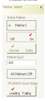
When in the or WCDMA measurement mode with the Random Access Channel with Zoom or Transmit Power Control with Zoom graph type, the following marker selections are available (Refer to the WCDMA Graph Type Dialog on page 4-48 for information on setting graph types):
